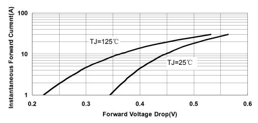
Fig.3-Typical Instantaneous Forward Voltage Characteristics
